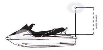
PWC's need to have a port (red) and a starboard (green) side light each showing an unbroken light over an arc of the horizon of 112.5°. If the design of the boat allows, a combination port and starboard light unit can
