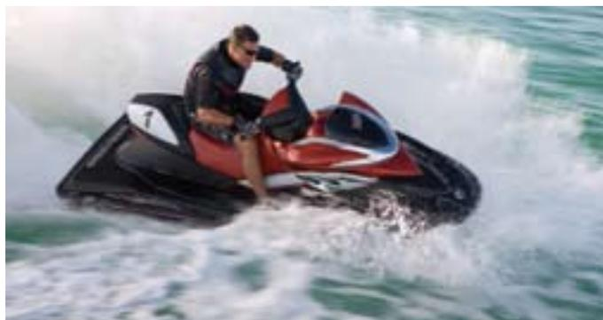
This connection between steerage and power is the most critical aspect to understand about operating a PWC and cannot be over-emphasised. Many accidents have occurred when a PWC operator has collided with objects or people after turning off the engine or reducing power.
