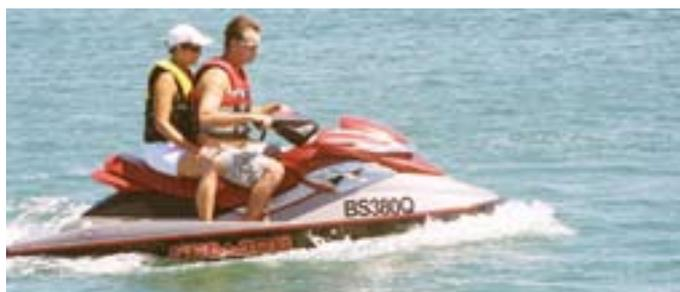
**Sub-planing** is medium speed. The bow of the PWC is out of the water, but the stern is forced deeper in the water which creates a larger wake.
