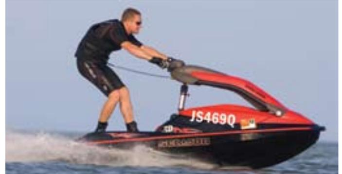
**Performance-orientated PWC (stand-up):** Featuring a hinged, adjustable steering column, the rider stands or kneels on a platform at the stern of the boat. These are often used for racing, and require skill and balance to operate. They can accommodate only one rider.
