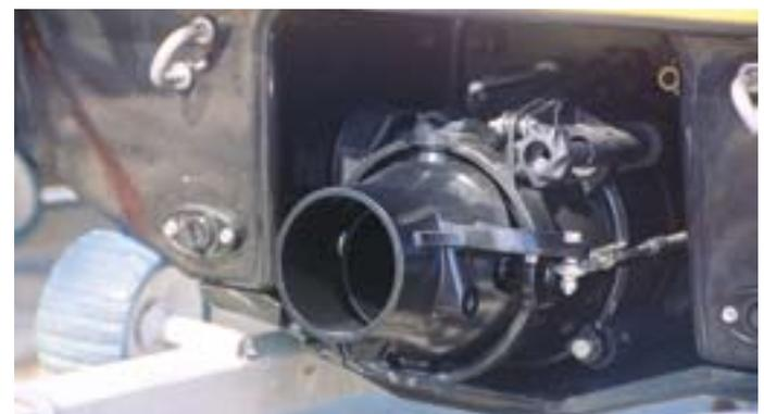
This jet of pressurised water propels and steers the craft when the throttle is engaged. Some newer PWC include 'off-throttle steering technology' which offers the craft limited manoeuvrability when the throttle is off.
