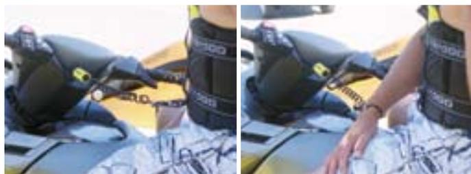
The safety switch works by attaching a lanyard between the operator and the switch. It is attached either to the operator’s PFD (above left) or their wrist (above right). If the lanyard is removed from the switch, then the engine will shut off.
