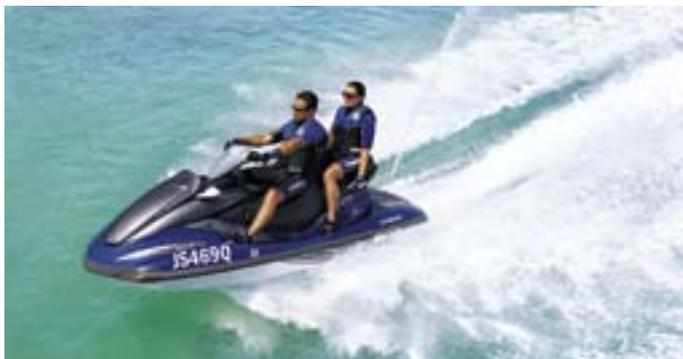
**Planing** is a faster speed where the bow and the stern of the PWC are level. The entire craft is skimming on top of the water, which creates a minimal wake.
